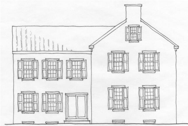
**Figure 34.** *These proposed new sliding doors do not follow the rhythm, scale and proportions of the existing primary façade and would not be recommended in the historic district.*
