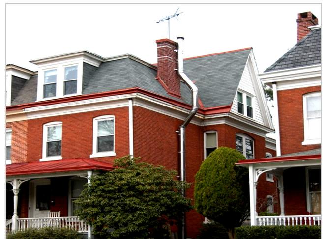
**Figure 33.** Example of inappropriate mechanical equipment installation. Stainless steel flue outside of chimney.
